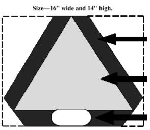
Shape—Equilateral triangle, one point up, points cut off, edges smooth, and corners slightly rounded.
